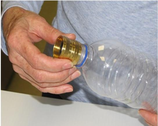
A double female hose connector is attached to 500 mL bottle. This small bottle contains the catching solution. About 100 mL of soapy water or commercial antifreeze solution can be poured into the small bottle to kill and preserved captured insects.
