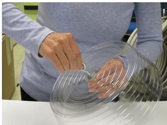
An eye bolt is screwed to a nut and a washer before attaching it to a plastic plant saucer. A hole at the center of the plastic saucer is made previously with a knife. The saucer protects the catching bottle from rain.
