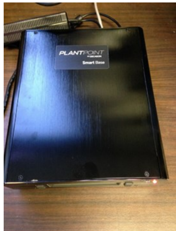
Figure 4. Base station computer generates a website that can be accessed online. This computer is used to control the network and create irrigation settings. The website can be customized to include information specific to the farm, sensor location, and output content.
