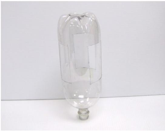
A 2 liter soda bottle is perforated with three rectangular holes (~60x100mm) on the periphery and a small hole at the center of the bottom. The upper part of the bottle becomes a funnel when the bottle is inverted, that conveys the insects to the catching bottle.
