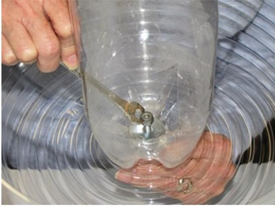
A washer and a locknut are screwed to fasten the soda bottle to the saucer.
